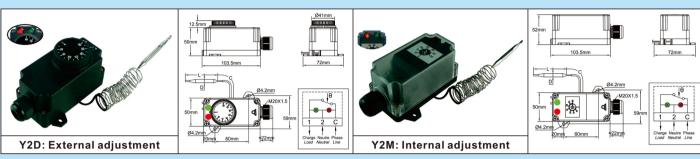
Housing: PC-ABS, fiberglass reinforced, UL94V0. High impact and UV resistance, with waterproof gasket on thermostat shaft for external adjustment types. Internal adjustment types have a PC transparent cover, to visualize the pilot lights and the set point adjustment.
