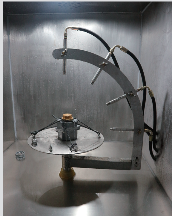
Enclosure during IPx9k test
