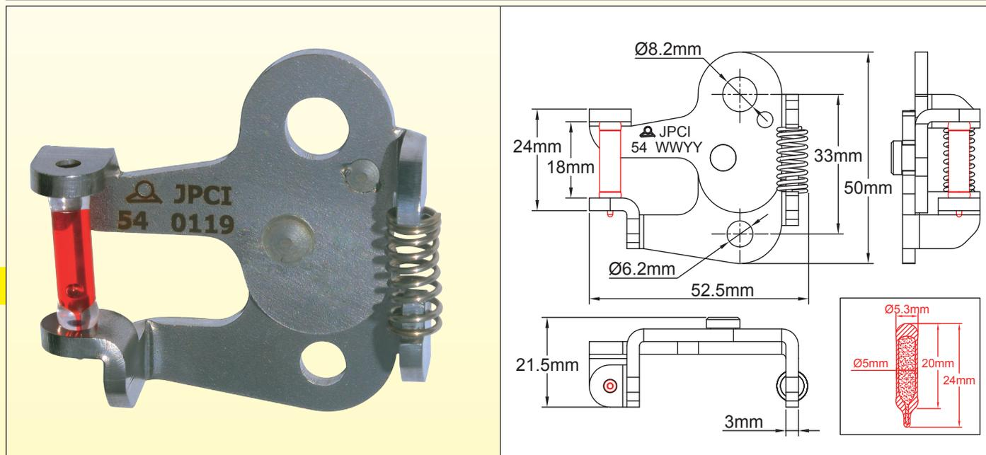
Made of 3mm thick galvanized steel, these reduction mechanisms are compatible with 20x5mm thermal glass bulbs. Their huge multiplying coefficient reduces the force applied to the thermal glass bulb to only 15% of that applied to the mechanism. The replacement of the glass bulb is simple and can be done without special tools. They withstand the 300 DaN overload during 5 minutes, and a minimal load of 0.4 DaN.
