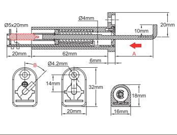
These mechanical thermal actuators are intended to close the fire dampers used on the ventilation ducts. Their large operating force unlocks the spring actuating the damper. Requiring no power supply, these devices are particularly simple and reliable. They are mandatory for all fire dampers to meet the NF-S 61.937 standard. Since thermal bulbs are not subject to creep, their periodic replacement is not necessary.
