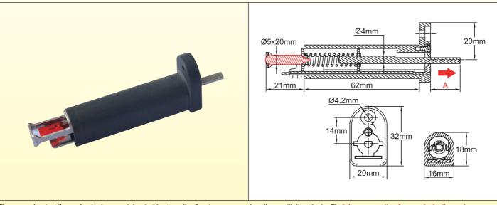
These mechanical thermal actuators are intended to close the fire dampers used on the ventilation ducts. Their large operating force unlocks the spring actuating the damper. Requiring no power supply, these devices are particularly simple and reliable.
