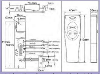
Used when the control boxes are located high or difficult to access. Allows remote start of control boxes, from up to 8 meters. Infrared control do not cause radio interference. Mounts on all control box models with window and terminal block (not possible junction boxes and Ground Fault Circuit Interrupter boxes). Current rating: 12A 250VAC.
