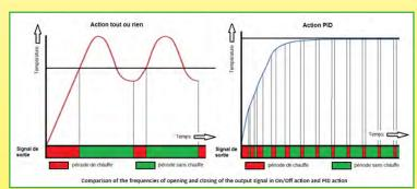
If the PID action can improve the control in a number of configurations, the drawback is that the output signal will cycle very quickly, which reduces the power relay life very extensively and requires in most cases to use solid state relays.
