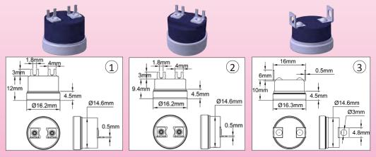
This disc thermostat is adapted to cable end mounting, with small size solder terminals and aluminum cup. It withstands silicone or epoxy filling. See page 93 for assembly method. Thermostat opens on temperature rise
