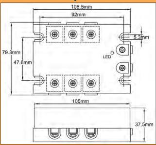
**Dimensions:** 108.5 x 76.3 x 37.5 mm Mounting: 4 holes M4, 48 x 92 mm spacing Operating voltage range: 24-440 V AC, 47 to 63 Hz Input signal: 3-32V DC, 12 to 25 mA current Voltage drop in open position (current flowing): <1.5VAC
