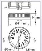
Intended for versions with room or capillary thermostats, this controller is equipped with internal lighting allowing by transparency a night viewing thermostat setting.
