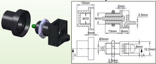
Enables the mounting of a manual reset thermostat on a face, with access to the reset push button by the orthogonal side. Sealed with the protection cap mounted. Access with a tool (EN60335-1 §22-10, §30.1). Requires a single 10mm drilling in the wall.
