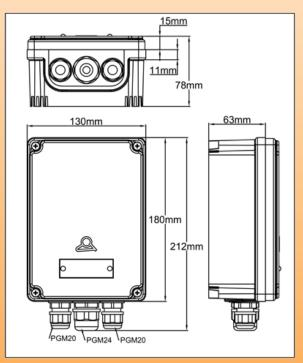
These sealed aluminum boxes are RAL 7015 epoxy painted. They have the same dimensions than the plastic control boxes, and use the same lids. They have the same external fixing pins than the other boxes, but they allow the mounting of single or three phase solid state relays of which the cooling is carried by the fins on the rear face.
