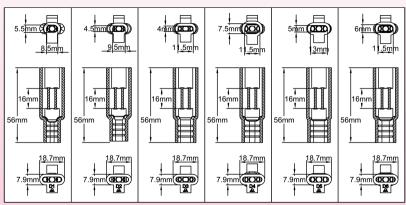
They allow the connection of heating cables on non-heating conventional conductors. When the assembly and filling are performed according to installation instructions, they provide an IP65 seal. Used with AWG15 wires (1.5 mm<sup>2</sup>) FEP insulated 300V, 300mm length (diameter 2.4 mm), equipped with a cable shoe and a tubular crimp terminal. After crimping non-heating wires, the connection to the control box is made with the M20x1.5 accessories with 2.4mm holes.
