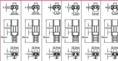
They allow the connection of heating cables on non-heating conventional conductors. When the assembly and filling are performed according to installation instructions, they provide an IP65 seal.
