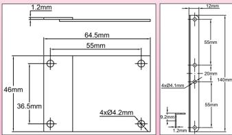
Coupling brackets for side-by-side boxes on the same heat-tracing stand
