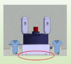
Without cross-wall. Allows use of the thermostat disc in most common applications. The low residual wall thickness greatly reduces the thermal inertia.
