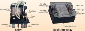
The relay or electromechanical contactor: The coil is made of a very large number of turns of a very thin copper wire. When a sufficient current goes through the coil, it produces a magnetic field that attracts the movable part and moves the reeds with electrical contacts. When the current no longer flows in the coil, the contacts return to their initial position thanks to a restoring spring.
