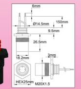
Anti-freeze thermostat with M20x1.5 front fitting
