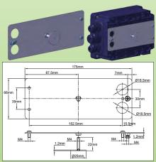
Designed for industrial heating blankets with thermal insulation. It consists of a 180x50mm stainless steel plate mounted at the rear of the Y8 box with the flexible heating surface in sandwich between the back plate and screw with a wide dia. 20mm head maintains the grounding continuity to the wall on which the soft heating element is mounted, while pressing the insulation
