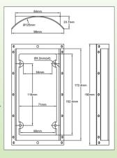
Model for diameter 125mm air duct
