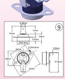
Anti-freeze thermostat, for trough wall mounting on junction or connection boxes, 6.3 x 0.8 tab terminals. Aluminum temperature sensing extended cup. Contact opens on temperature rise.
