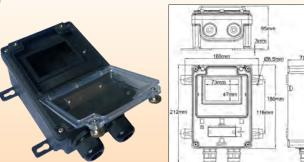
Allows mounting of a circuit breaker type Merlin Gerin Multi 9 (UL, CSA, IEC) and equiva-lent European ranges Vigi C60 or C60 (72mm maximum width = four 18 mm modules), or electronic controllers described in this catalogue
