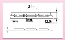
Although more expensive than the traditional aluminum tapes, this solution is perfectly temperature-resistant, and allows fast and durable assembly, and the ability to reposition or replace cables. It can also cost effectively replace the hose serrage. Tape having evenly spaced tabs. These foldable tabs allow to set the heating cables at a constant distance.
