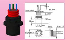
3 wires Pt100 sensor in an anodized aluminum bolt. To measure the temperature outside of cabinet: can be screwed directly to the rear outputs M20 thread or to the cable gland outlet board.
