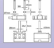
Only for adjustable bulb and capillary thermostats. This switch enables an off/off two poles action 16A 250V, activated when the knob is turned back to its minimum angle position. For foot print reasons, this option cannot be mounted with ranges above 320  $^{\circ}$  C, nor on the three pole thermostats.
