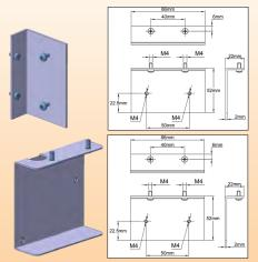
SSR mounting plate on electronic front board . Fits all electronic controllers with SSR output.in this catalog Material: aluminum.
