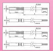
3 conductors set, 300V FEP insulation, for non heating output. Equipped with cable shoes at one end and a tubular connector crimped at the other end, they save time on site by limiting cutting, stripping and crimping operations.
