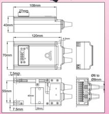
Enclosure: Light cream color PC-ABS (RAL1010), small footprint, can be hand held or wall mounted Ingress protection rating: IP54 (IEC 60529)
