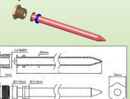
External diameter 8 mm, internal 6.5 mm, with flat seal bearing. Mounting with 1/4" BSPP brass nut and a flat internal fiber gasket (included). These cheap pockets (no solder nor brazing between the joint and the tube) are designed for dia. 6mm bulb or sensor insertion.
