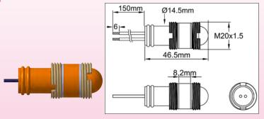
This pilot light shows the presence of 230V at the end of a parallel heating cable. It is screwed on the insulation plate, or on any other outlet with M20x1.5 thread. The set includes an indicator light, two stainless steel washers and two M20x1.5 nuts
