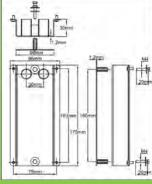
It consists of a stainless steel rear bracket mounted on the back of the Y8 box , keeping the heating element 30mm aside from the heating surface, and a 180x50mm stainless steel back plate. The small width of the back plate enables the support to keep its flexibility. The wide 180 mm length allows a strong fastening on the box.
