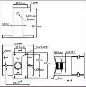
Can also be used for flat surface or a wall mounting, using the two dia. 8mm holes 80 mm spacing.
