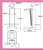
Intended for use with sealed connection sleeves types A, C, D, E, F, G. This stand keeps the pieces
