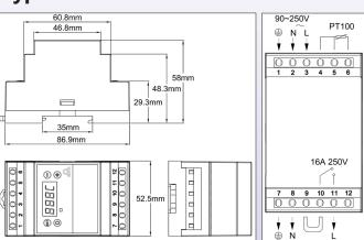
This electronic temperature controller with the simplest and instinctive end user setting, was designed for simple incorporation inside cabinets with DIN rail mounting, and to be used by not highly trained operators.
