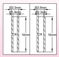
Allows in-line connection of leads with different gauges, including spiral heating wires on fiberglass cores. The pods must be protected by a heat shrink sleeve if a sealing connection plug with silicone filling is not used.
