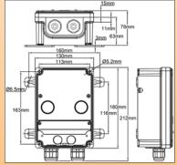
$3\times16A$  (AC1), 250V, Ultimheat terminal block with 5 terminals 2.5 mm² screws and 5 screw terminals 6 mm². Red indicator light for power supply and output green light (250V), transparent lid. Shunts: see page 74
