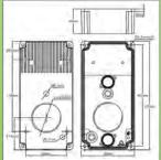
It includes aluminum housing, 4 screws, and the housing gas-
