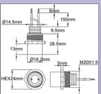
2 wires NTC in an anodized aluminum bolt
