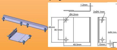
FFor side by side mounting of box equipped with a weather protected fan on an other box of the same dimensions
