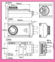
Enclosure: Light cream color PC-ABS (RAL1010), small footprint, can be hand held of wall mounted lngress protection rating: IP54 (IEC 60529)
