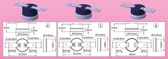
Anti-freeze thermostat, for mounting on heating cable end under double wall shrinkable sleeve, with  $6.3\times0.8$  horizontal tab terminals, for faston connectors or soldering. Aluminum temperature sensing cup. Contact opens on temperature rise.
