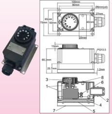
Housing: IP65, 100 x50 x 69 mm, PA66 30%FG, UL94V0. High impact and UV resistance, with waterproof gasket on thermostat shaft (1). Mounted on a SUS304 stainless steel wall mounting plate which keeps temperature (2).
