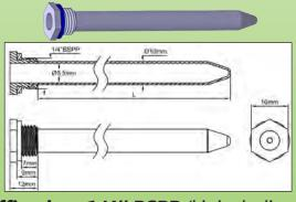
External diameter 10 mm, internal 8.5 mm, with 1/4"BSPP brazed joint and a flat internal fiber gasket (included). Flat seal bearing under the joint hexagon. These pockets are designed for dia. 8 mm bulb, sensor and thermal cutoff insertion. Putting some thermal compound on the sensors improves the response time. The kit includes: pocket, fiber gasket. Stainless steel versions on custom manufacturing
