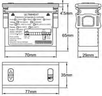
Mini-sized and integrated intelligent controller, with very simple end-user interface: Change of set point is made without password, with up and down keys.
