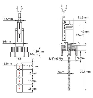
**Main uses:** <u>Large quantities applications</u> in flow detection in low voltage electronic circuits. The most economical model. Recommended mounting position is on horizontal pipes. Can be mounted in any position with a small drift in the calibration because of the paddle weight. Can be used on **15 to 100mm diameter** water pipes.
